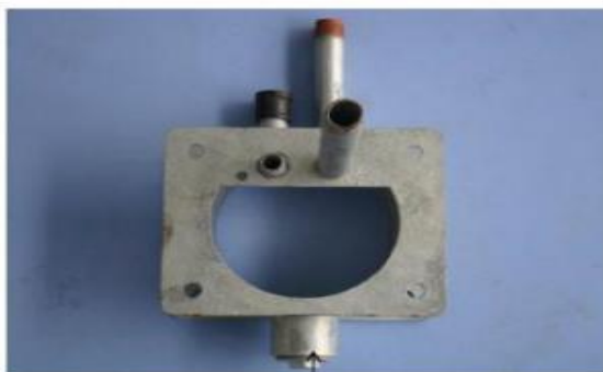
Inlet for rooftop rainwater harvesting
